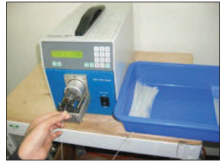
▲ Fig. 4 CMC semi-automatic stripper assures quality with precision and stable tolerance control.
