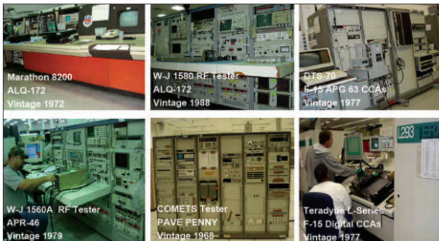
▲ Fig. 2 Legacy testers replaced by VDATS.
