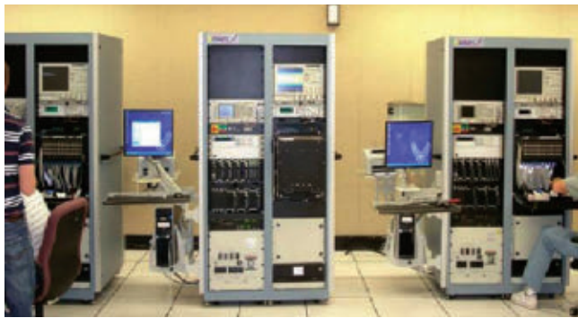
▲ Fig. 1 Multiple VDATS with RF Auxiliary Unit at Warner Robins Air Force Base.
