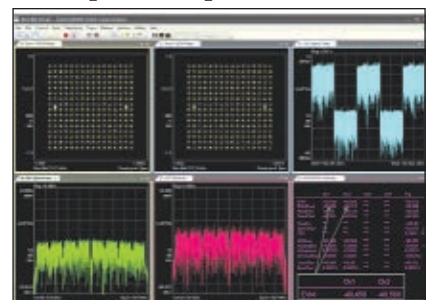
▲ Fig. 7 VSA MIMO demodulation using VSA software on the 13 GHz digital oscilloscope.
