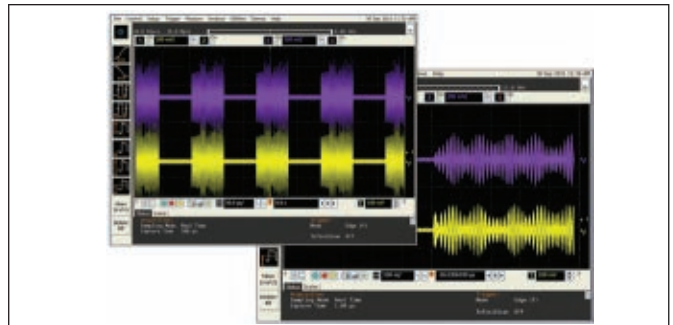
▲ Fig. 6 Time measurement of the master/slave AWG MIMO waveforms.
