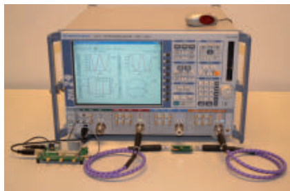
▲ Fig. 1 NM310S starter kit connected to a Rohde & Schwarz ZVA24.
